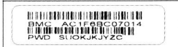
Figure 1: BMC barcode label displaying BMC MAC address and ADMIN user unique password
